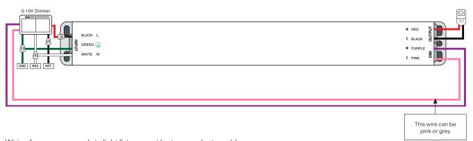
Wiring from power supply to light fixture must be two conductor cable. \\
